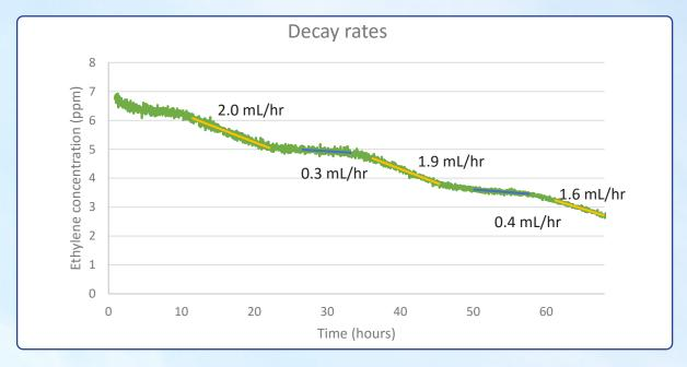
Decay rates in milliliter per hour determined for when the air cleaner is on (yellow) or off (blue). The decay rate in percentage is between 1.5~% - 2.0~%.
