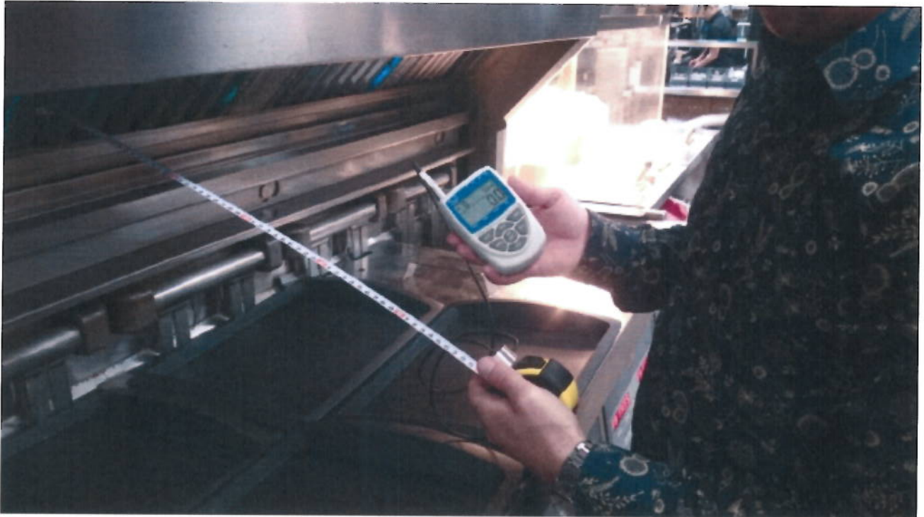
Figure 4: Filter and light on, measurement at 60cm distance, with oil cover seen
